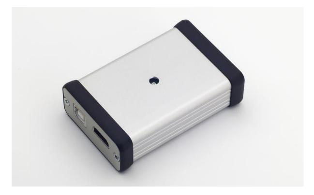
The third device type that is needed, is a convertor from SDI to HDMI, as the screens above do not possess the ability to accept SDI signals. We use a Black Magic design UP/DownCross HD convertor to achieve this conversion.
